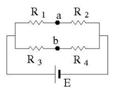
What is the necessary value of  $R_4$  such that the potential difference between points a and b is 0?\_\_\_\_\_
