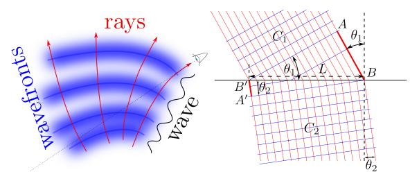
the media 1 with speed  $c_1$  as for it to travel from B' to A' in the media 2 with the speed  $c_2$ , so  $\frac{|AB|}{c_1} = \frac{|B'A'|}{c_2}$ . If the distance |B'B| is L, then  $|AB| = L \sin \theta_1$  and  $|B'A'| = L \sin \theta$ . So we get
