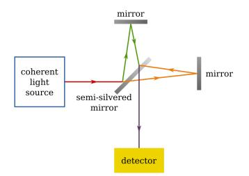
**Figure 1.** A Michelson interferometer uses the same principle as the original experiment. But it uses a laser for a light source.
