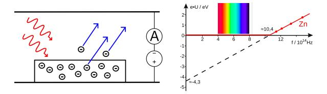
One shines light on a metal plate. The metal plate is on one plate of a parallel plate capacitor, see figure. We can apply voltage to the plates of the capacitor and measure current. We also can control the frequency/wavelength and intensity of the light.
