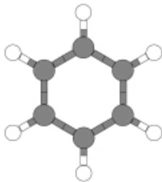
Figure 33: Benzene molecule in the ground state. It has two fully-symmetric vibrational modes: In the breathing mode, the carbon and hydrogen atoms move radially together in the plane of the molecule; in the beating mode they also move radially, but in opposite directions.
