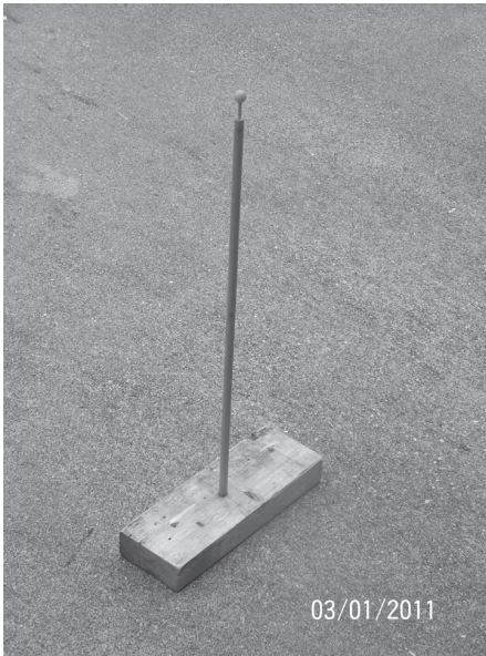
Figure 7.3 Device for measuring the elevation angle of the Sun above the horizon.
