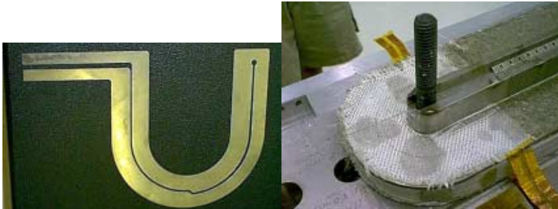
Figure 7. Quench heater: a) foil heater; b) heater installed with S-glass insulation to coil and mica paper insulation to rib.
